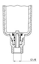
To avoid the discharge of condensate, the drain. the operator mechanism should be turned clockwise to completely close
