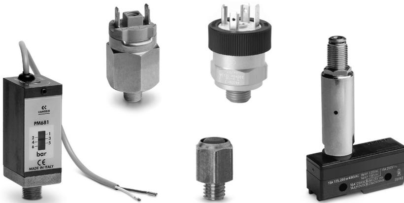
A regulating screw, which can be adjusted using a small screwdriver, allows the switch to be set to the required pressure. The calibrated diaphragm enables an electrical signal to be generated or inhibited depending on the pressure set.
