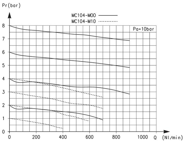
Flow diagram for model: MC104-M00
