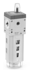
The operating principle is based on the adsorption characteristic of the filtering element which is composed of extremely porous fibers placed on different layers. These fibers create a cross-linked and are thus able to adsorb wet parts and contaminants remaining in the passing air, for example oil vapours/smokes, as well as odours generated from these contaminants.
