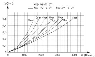
\* Reference diagram for models with filtering element = 0.01  $\mu m$
