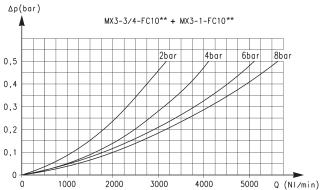
\* Reference diagram for models with filtering element =  $0.01 \mu m$
